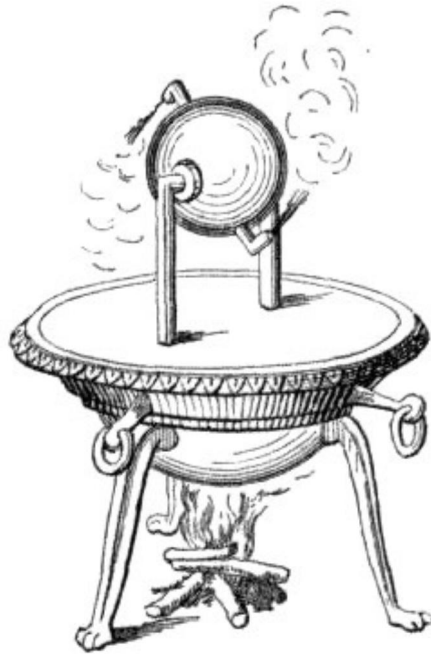
Figure 3 The aeolipile of Heron of Alexandria
